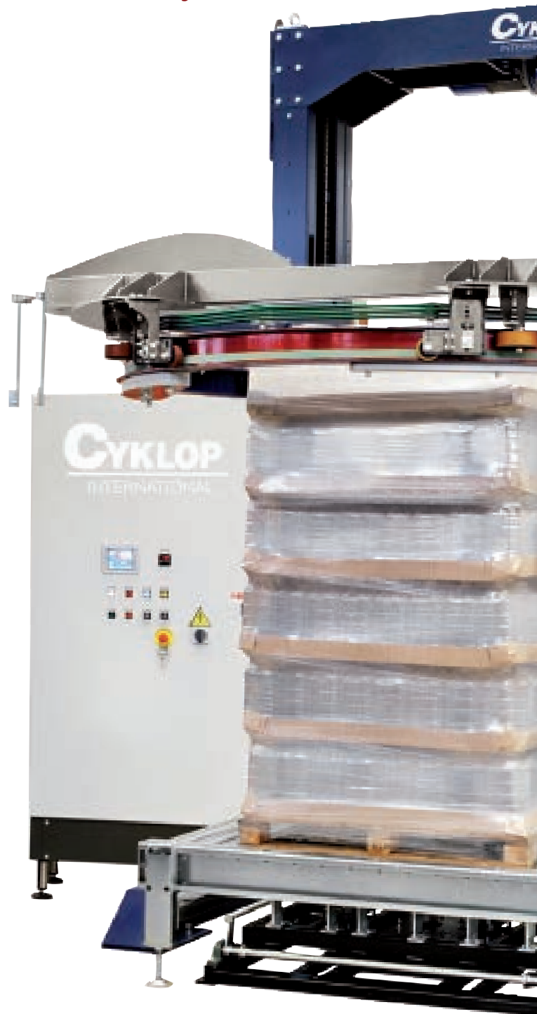
External pre-stretch dry system.
